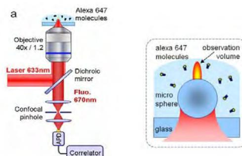
**Fig. 1:** Left panel: Sketch of the experimental configuration. Right panel: close-up on the microsphere.
