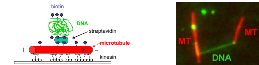
Fig.1 Diagram of DNA attachment to a kinesin-driven microtubule by streptavidin and biotin.
